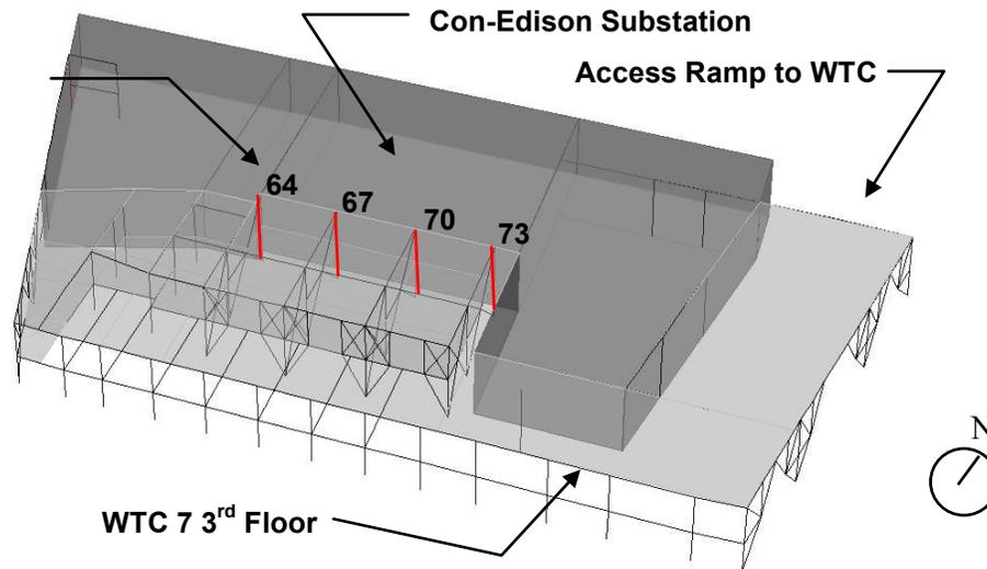
Figure L-4. Con Ed substation location relative to the WTC 7 building.
