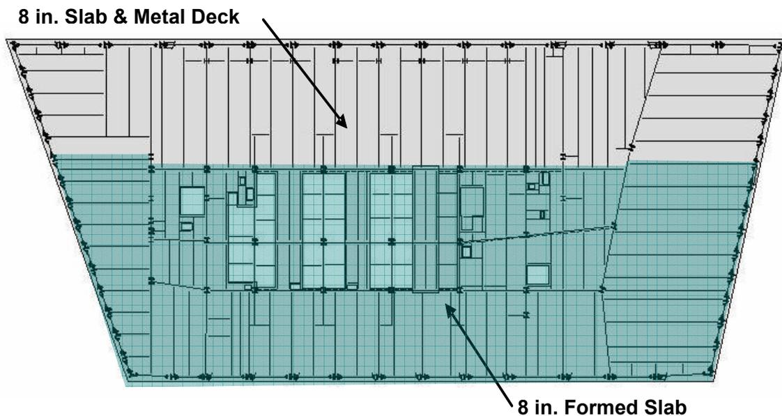
Figure L-13. Floor 7 plan.
