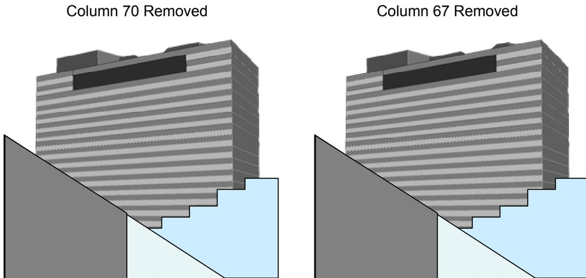
Figure L-42. Geometry changes for removal of columns 70 and 67.
