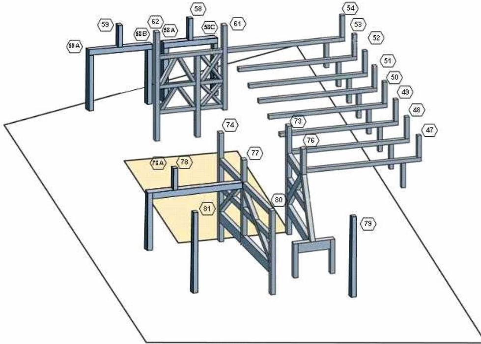
**Figure L–18. 3D schematic view of transfer trusses and girders between Floors 5 and 7.**
