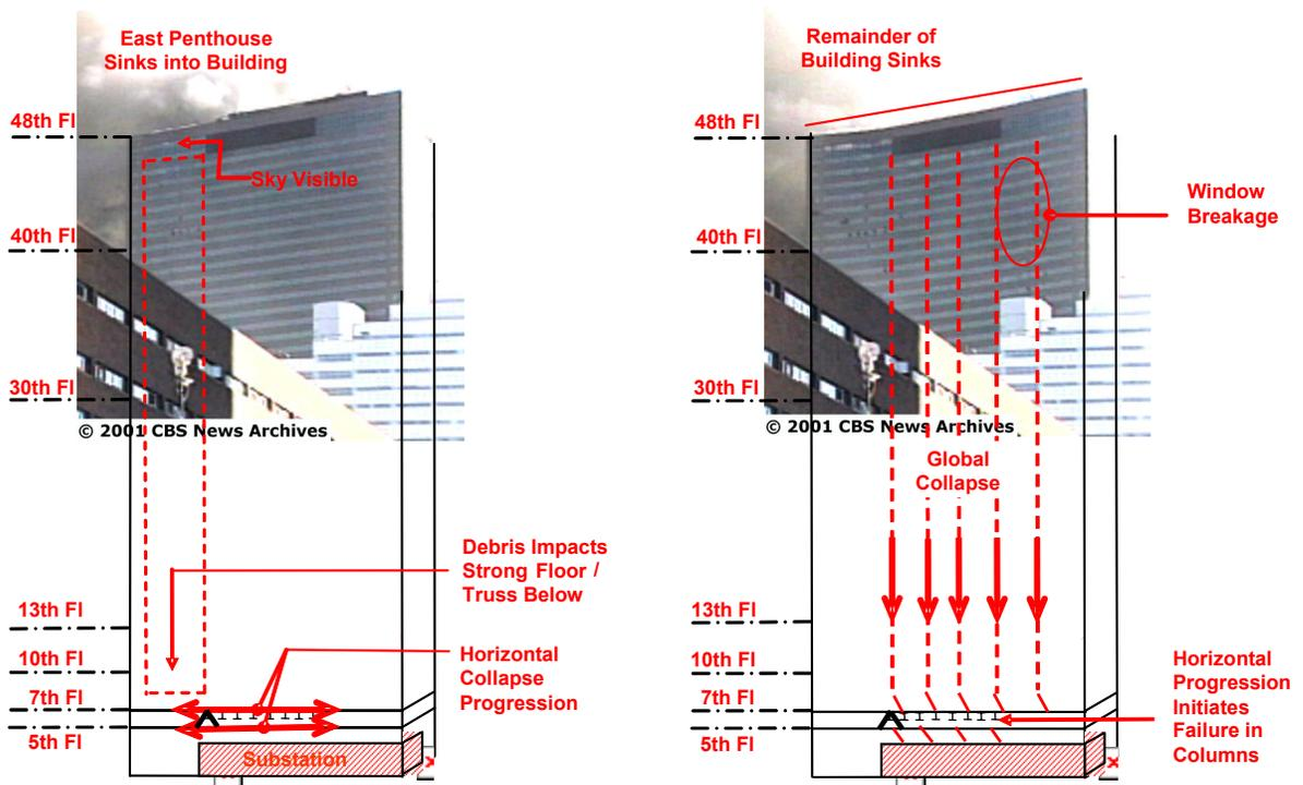
Figure L-34. Horizontal progression to the west side of WTC 7.
