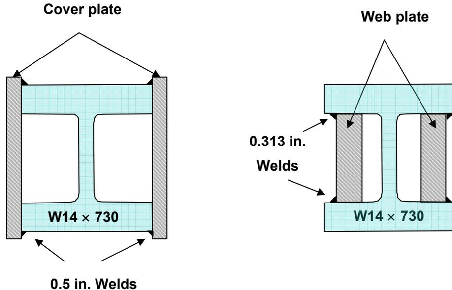
**Figure L-17. Typical built-up column details.**
