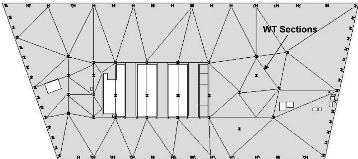
Figure L-11. Floor 5 diaphragm plan.
