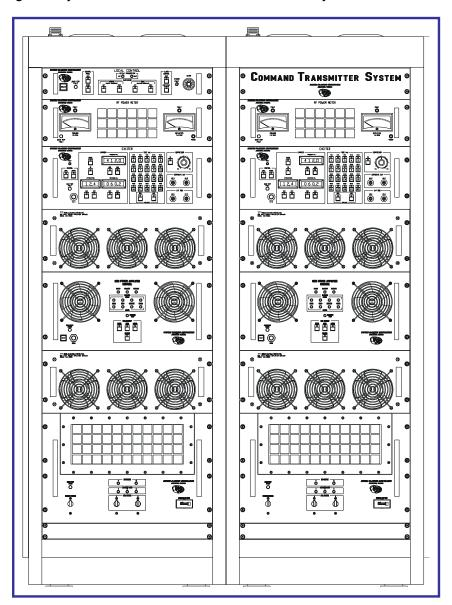
State-of-the-art CMOS micro-controllers provide full fault detection and reporting. High-power ferrite isolators allow full-power operation with antenna VSWRs up to 2:1. The HPA is designed for graceful degradation, which allows high-output power operation even with several amplifier modules inoperative. As an optional feature, each HPA sub-system is provided with an RF switch matrix that allows real-time replacement of HPA units.
